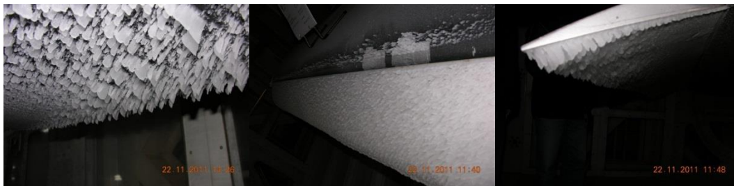
Figure 79 - Typical ice shapes in CIRA IWT wind tunnel
