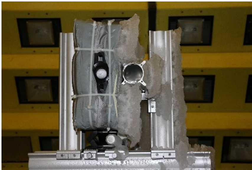
Figure 59: Illustration of fog on the collecting lens
